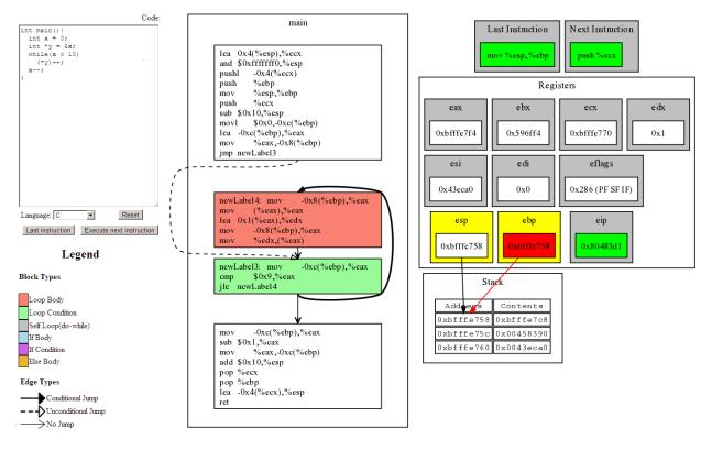
Figure 1: Simple while loop running through Frances-A.
